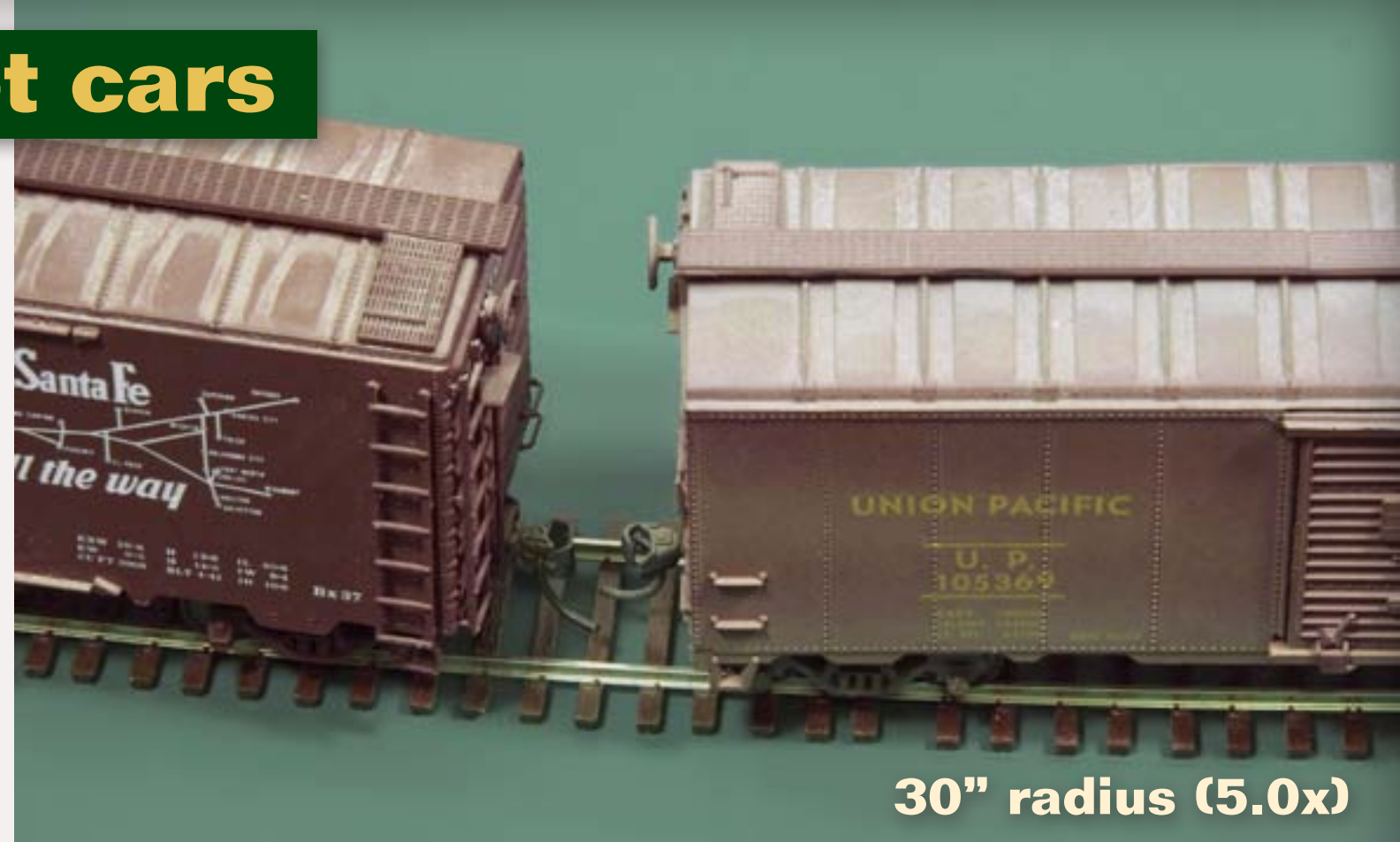
FIGURE 10: As the 5.0x guideline suggests, the coupler alignment on a 30" curve essentially matches that of straight track with 40 ft boxcars.
