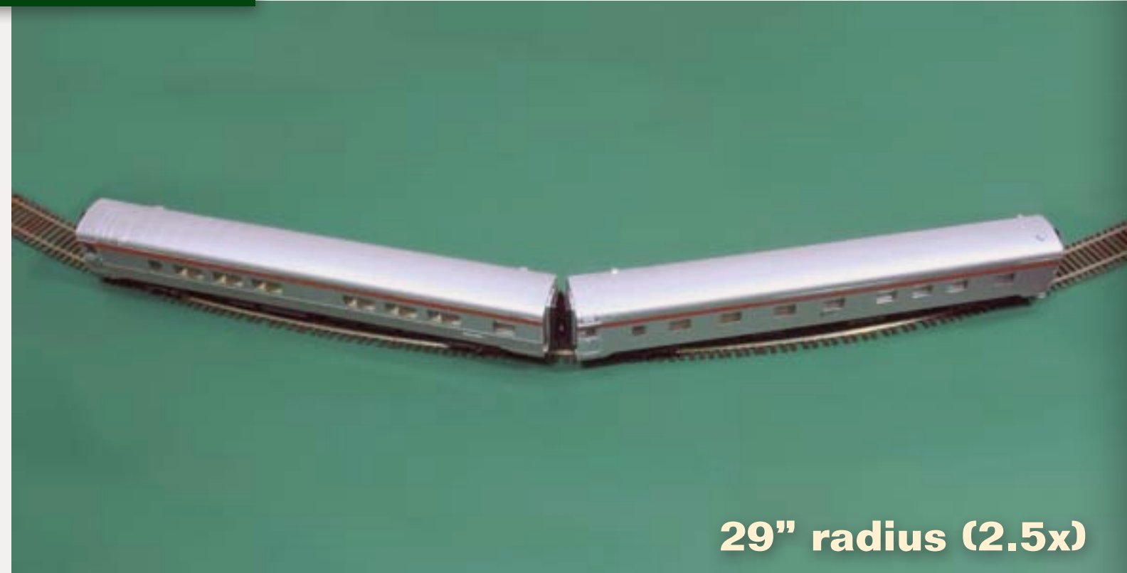
FIGURE 22: At the 2.5x radius, the cars finally will couple. They also track reasonably well at this radius, but they look totally unrealistic.
