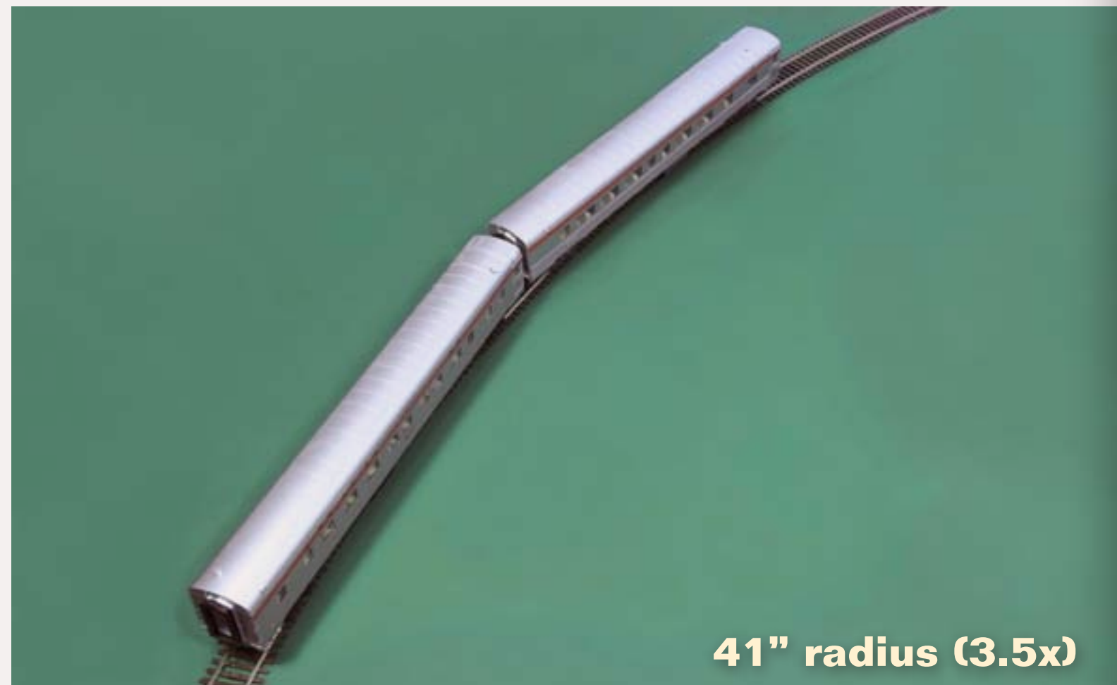
FIGURE 24: Upon reaching the 3.5x radius, the 80 foot cars look noticeably better when viewed from inside the curve.
