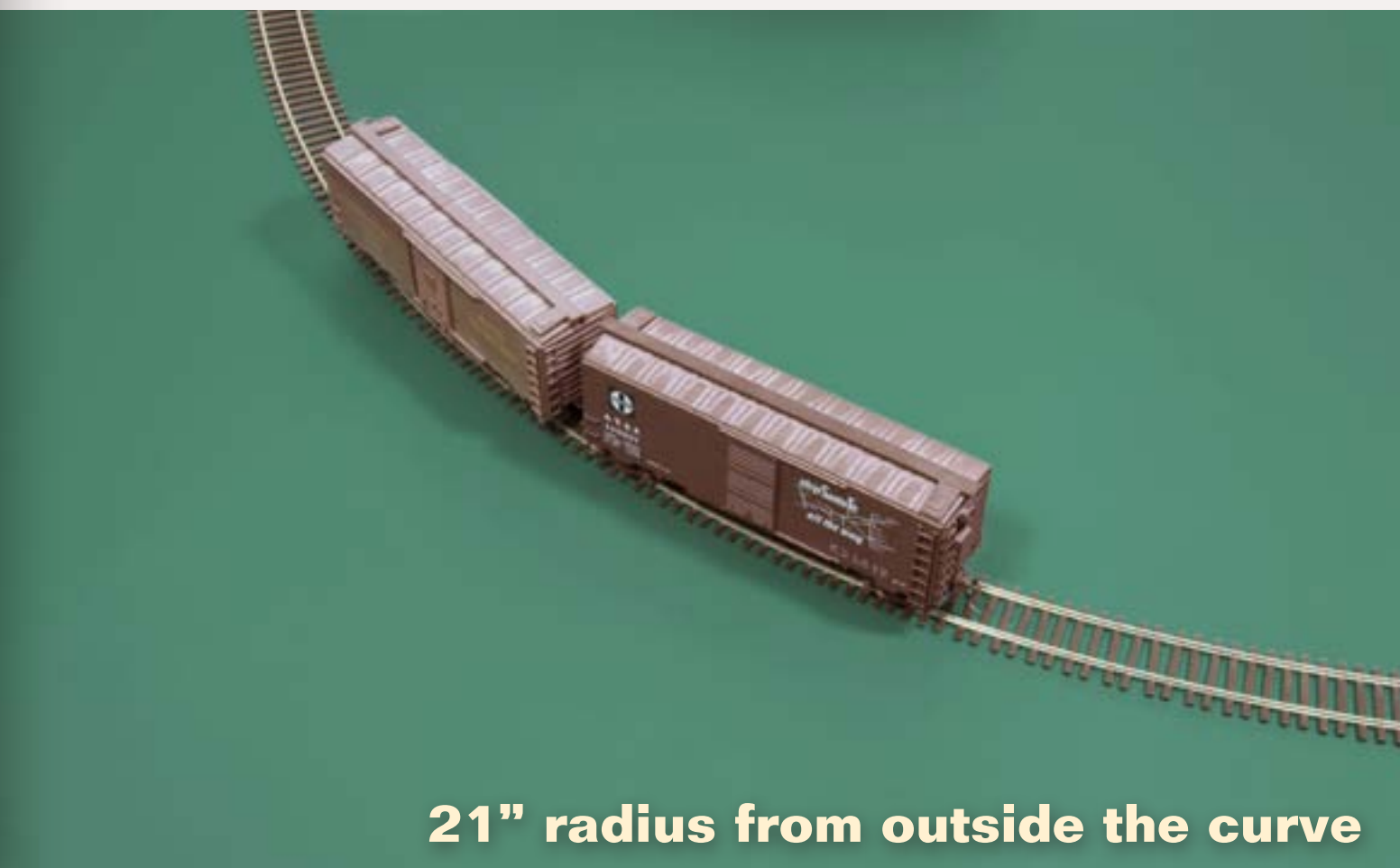
FIGURE 11: Here's a side-by-side comparison of a 3.5x radius curve when viewed from both inside and outside the curve.
