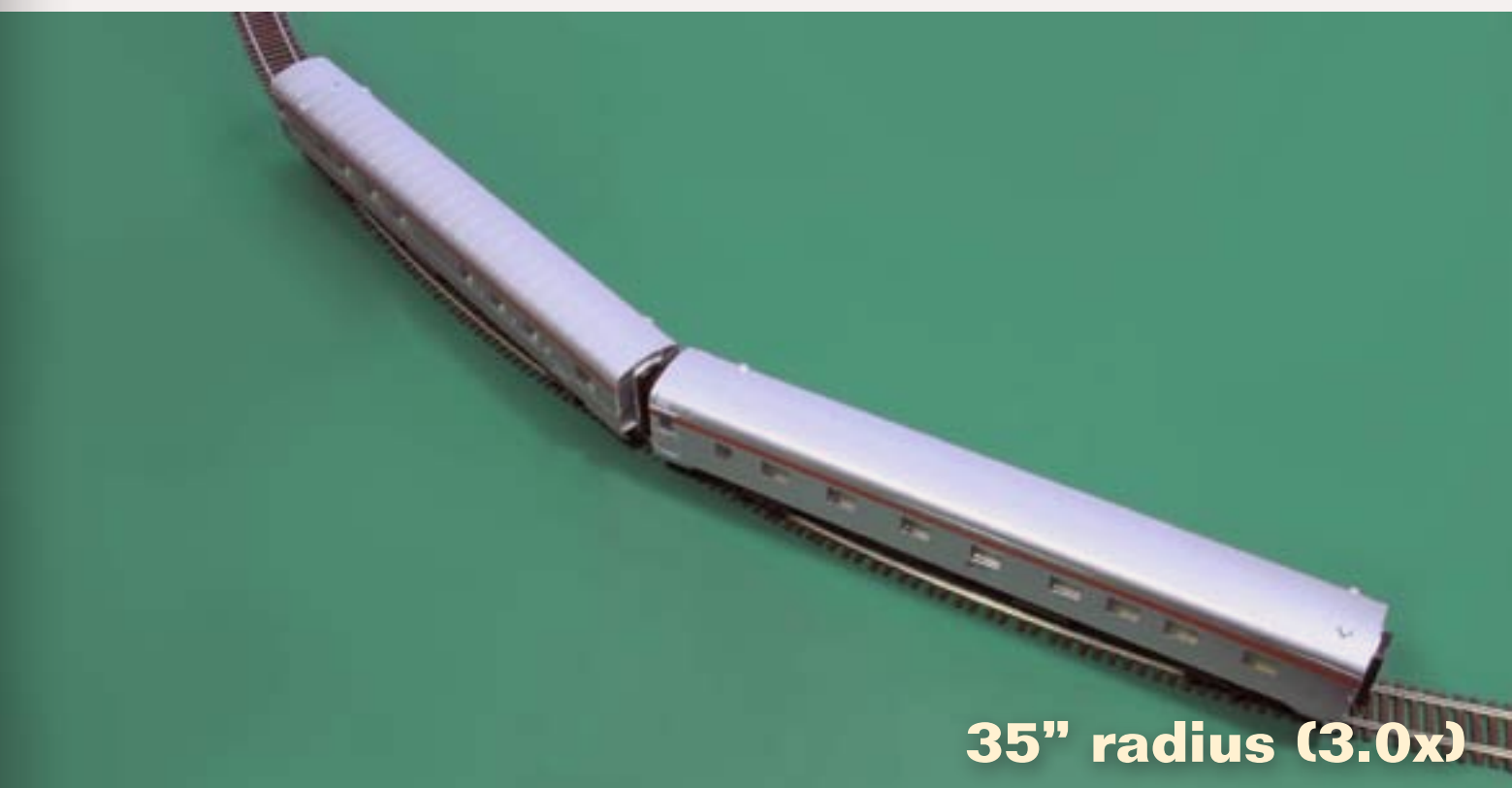
FIGURE 23: Once we reach the 3.0x radius, the cars roll very freely, with no tracking problems, although the overhang is still excessive.
