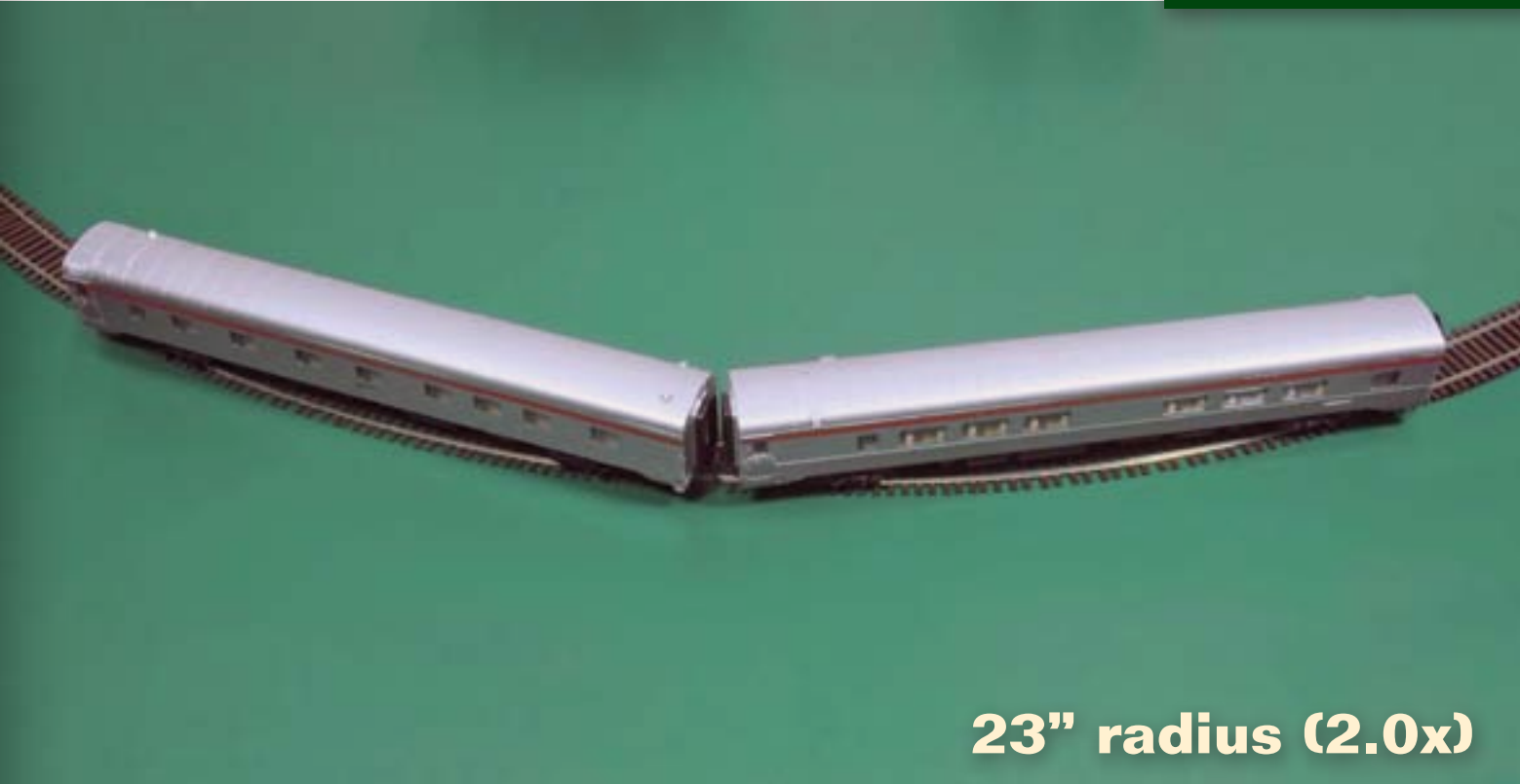
FIGURE 21: These 80 foot cars just barely stay on the track at the 2.0x radius, and fortunately there's no underbody detail in the way of the truck rotation. Most commonly, the trucks hit underbody detail or corner steps when the curve radius becomes too sharp. Also at this radius, the cars will not couple (the diaphragms are in the way).
