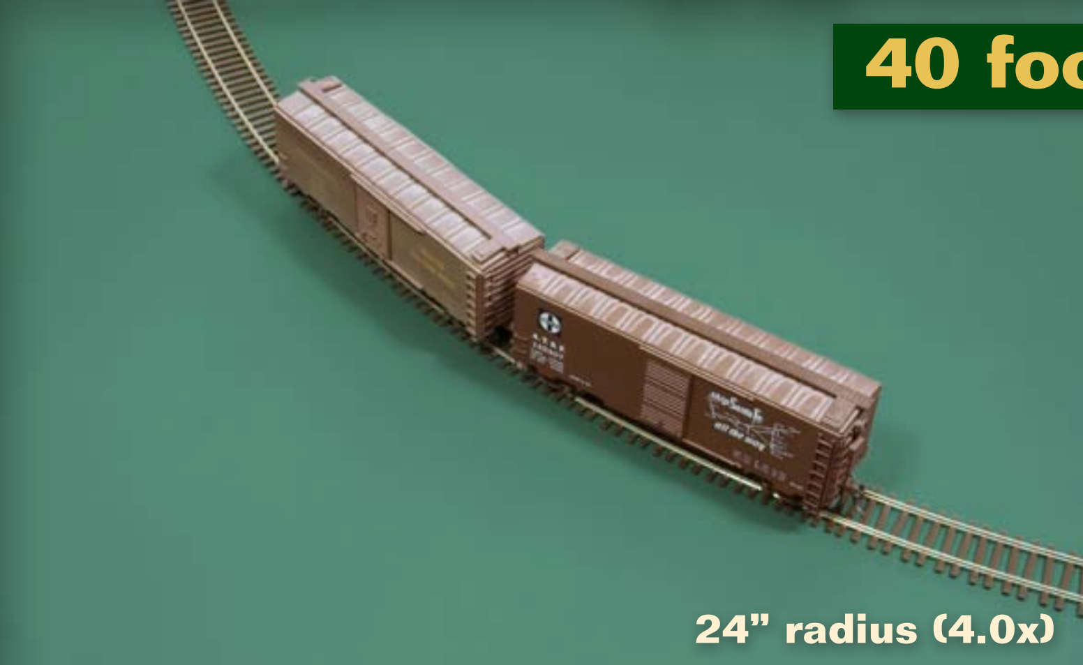
FIGURE 9: Once again as predicted, the cars look realistic at the 4.0x radius curve when viewed from the outside of the curve.
