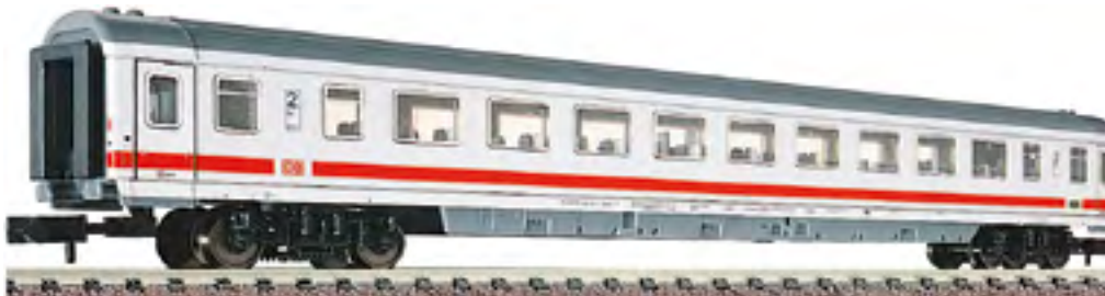
2nd class IC/EC high capacity wagon type Bpmz 295.5, DB AG.
