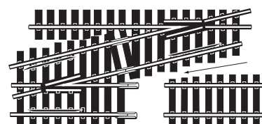
Fig. 1 Trim sleepers to fit
