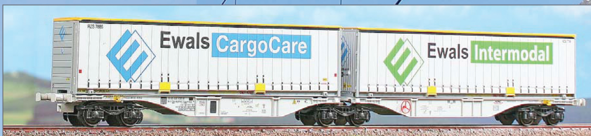
Carro intermodale Tipo Sggrss '90 bimodulo HUPAC caricato con due casse mobili "Ewals" ed "Ewals Intermodal" Container wagon Type Sggrss '90 HUPAC with two "Ewals" and "Ewals Intermodal" swap bodies Containerwagen Typ Sggrss '90 Doppelmodul der HUPAC mit "Ewals" und "Ewals Intermodal" Wechselpritschen
