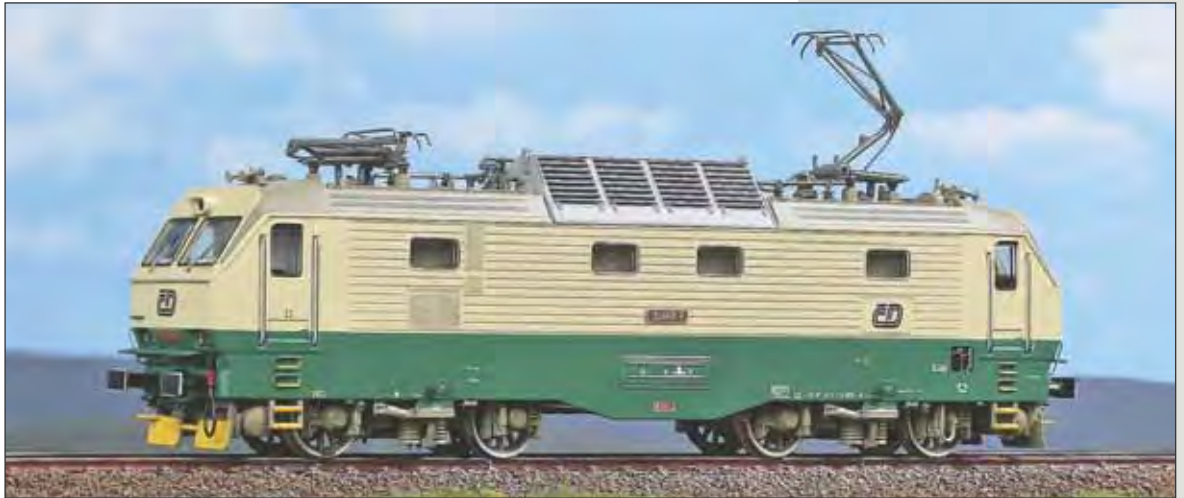
Locomotiva Classe 151 006 delle Ferrovie Cechе ČD per treni intercity. Class 151 006 locomotive of the ČD (Czech Railways) for intercity trains. E-Lok Baureihe 151 006 ČD (Tschechische Eisenbahnen) für Intercity-Züge.
