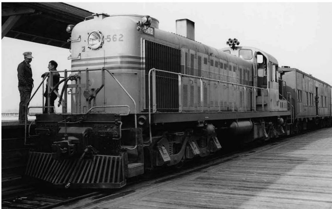
Canada's Pacific Great Eastern RSC-3 No. 562 leads converted troop sleepers. Notice the steam locomotive-style pilot. PGE's eight RSC-3s were later rebuilt with two-axle B trucks. PGE was renamed the British Columbia Railway in 1972 (later BC Rail) and was a large user of Alco and MLW locomotives. Jay Williams collection
