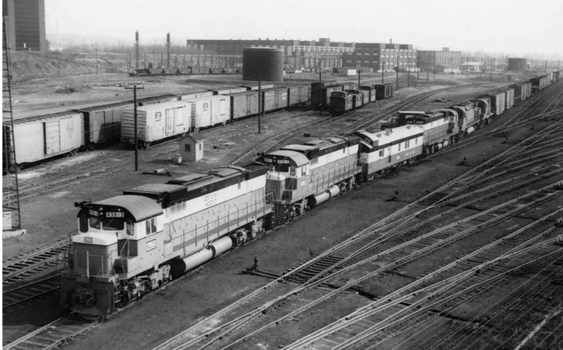
Alco's C-430 demonstrators operate with its dynamometer car (acquired from the Nickel Plate Road) on a Delaware & Hudson freight at Colonie, New York, on April 1, 1967. Alco's most powerful four-motor diesel had few buyers. Yet, like many of Alco's later diesels, the few that were built generally enjoyed long working lives. Several are still active in 2009. Jim Shaughnessy
