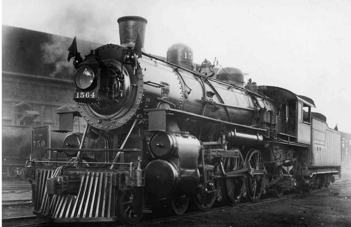
Chicago & North Western's Class E Pacific No. 1564 was built by Alco's Schenectady works in July 1911. The varnished wooden "cow-catcher" pilot was still a standard feature on road locomotives of the period. As built, this locomotive had 75-inch drivers, 25x28-inch cylinders, the boiler operated at 185 psi, and it weighed 154,500 pounds. It carries green flags and markers, which would have been used for the first or advanced section of a passenger train under timetable and train order rules. Chicago & North Western Railway photo by Christie, author collection
