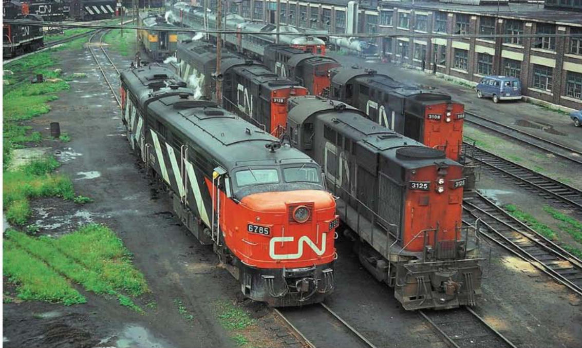
Toronto's Spedina Yard contains a host of Canadian National 251-powered MLWs on June 19, 1976. On the left is a pair of passenger-service FPA-4s; on the right are several RS-18s—MLW's equivalent to the RS-11. Don Marson
