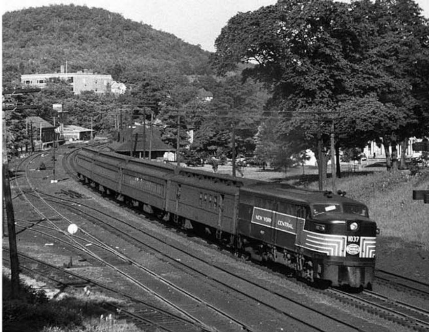
Photos of New York Central FA-1s on passenger trains are very rare. In October 1950, FA-1 No. 1037 leads train No. 48 on the Boston & Albany at Warren, Massachusetts. Because FA-1s were not equipped with steam generators, they could be assigned passenger runs in warmer months, but few railroads made a habit of doing so. Warren St. George, courtesy Robert A. Buck/Kenneth J. Buck collection
