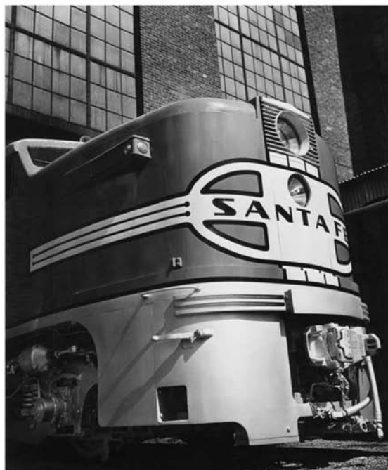
Right: Santa Fe No. 51 was the first Alco PA, a locomotive symbolically assigned Alco build number 75,000. After tests on the Lehigh Valley, it was painted in the famous warbonnet design and delivered to the Santa Fe for passenger service. Santa Fe photo by Jacob Lofman, W. A. Lucas collection, Railroad Museum of Pennsylvania PHMC
