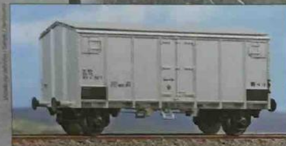
Carro refrigerante FS Tipo Hg, livrea alluminio. Type Hg refrigerator wagon of the Italian Railways, aluminium livery. Kühlwagen Typ Hg der FS, Aluminiumlackierung.
