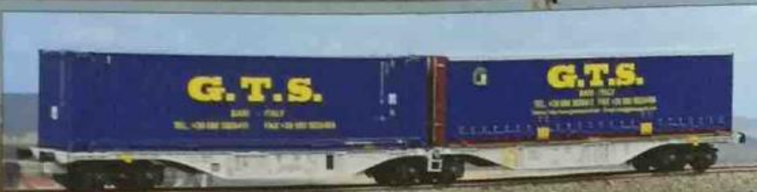
Carro intermodale Tipo Sggnms '90 binucleo noleggiato "GTS Rail" con carico di casse mobili. Container wagon Type Sggnms '90 hired by "GTS Rail" with swap bodies. Containerwagen Typ Sggnms '90 Doppelmodul vermietet an "GTS Rail" mit Wechselpritschen.
