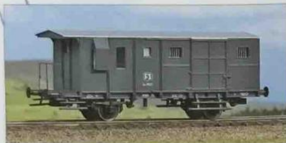
Bagagliaio FS per treni merci Tipo Dm, livrea grigio ardesia. Type Dm luggage car of the Italian Railways, slate gray livery. Güterzuggepäckwagen Typ Dm der FS, schiefergrau Lackierung.
