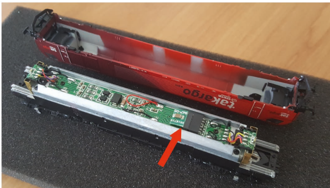
3. Install the decoder of your choice. Follow the manufacturer instructions.
