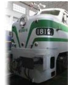
Diesel-electric locomotives are in principle electric locomotives with electrical generators that are powered by diesel engines. The diesel locomotive is generally driven at constant Driving notches subject to the speed of the locomotive. Therefore the noise generated changes (driving) step by (driving) step. The quiet electric motor can hardly be heard over the noise of the diesel powered plant. Most diesel-electric locomotives have 4 to 8 throttle notches.
