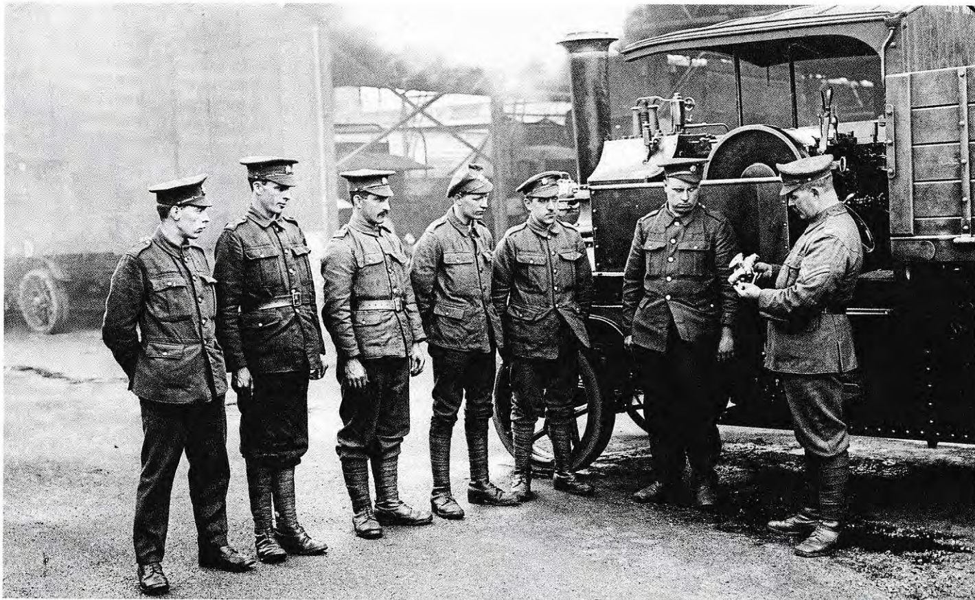
An ASC instructor has been advising the class of the differences between a traction engine and a Foden steam wagon. In his hands, he is holding an injector and is presumably using this to explain to the group of soldiers how such a device works. IWM - HU 069751
