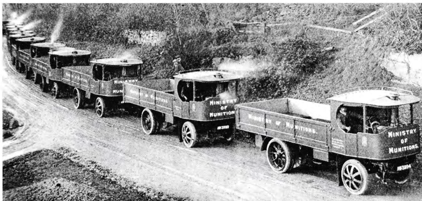
The caption for this photograph in Sentinel's house magazine Sentinel Transport News was 'Sentinel Steam Waggons undergoing official test before delivery to the Government'. The firm's Standard type wagons were supplied to the Ministry of Munitions from January 1918 onwards, with this image being taken in April 1918. These were therefore probably within the range of works numbers 1828-1842 inclusive. COURTESY TONY THOMAS
