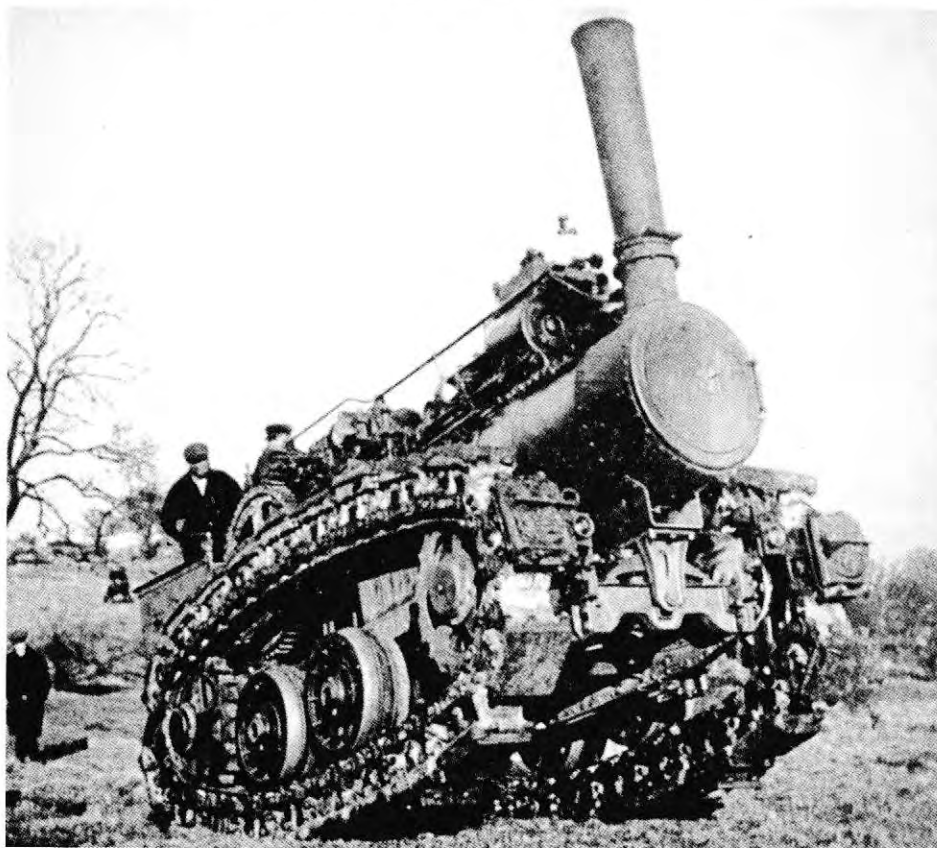
The Yukon chain track tractor of 1909 was important in the development of other similar machines.
