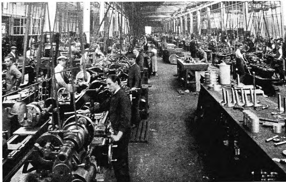
Badged men turning aircraft components at Ruston & Hornsby in 1917.
