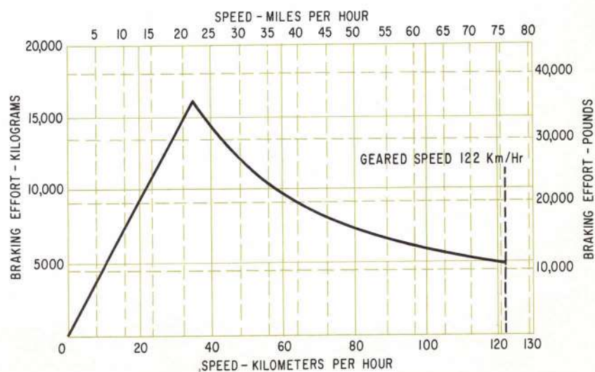
Braking Effort Characteristics with 1016 mm (40") Wheels and Basic 92:19 Gearing.
