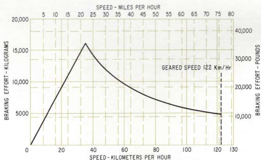
Bracing Effort Characteristics with 1016mm (40") Wheels and Basic 92:19 Gearing.
