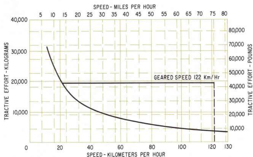
Tractive Effort Characteristics with 1016mm (40") Wheels and Basic 92:19 Gearing.
