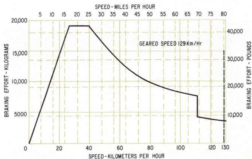
Braking Effort Characteristics with 1092 mm (43") Wheels and Basic 65:18 Gearing.
