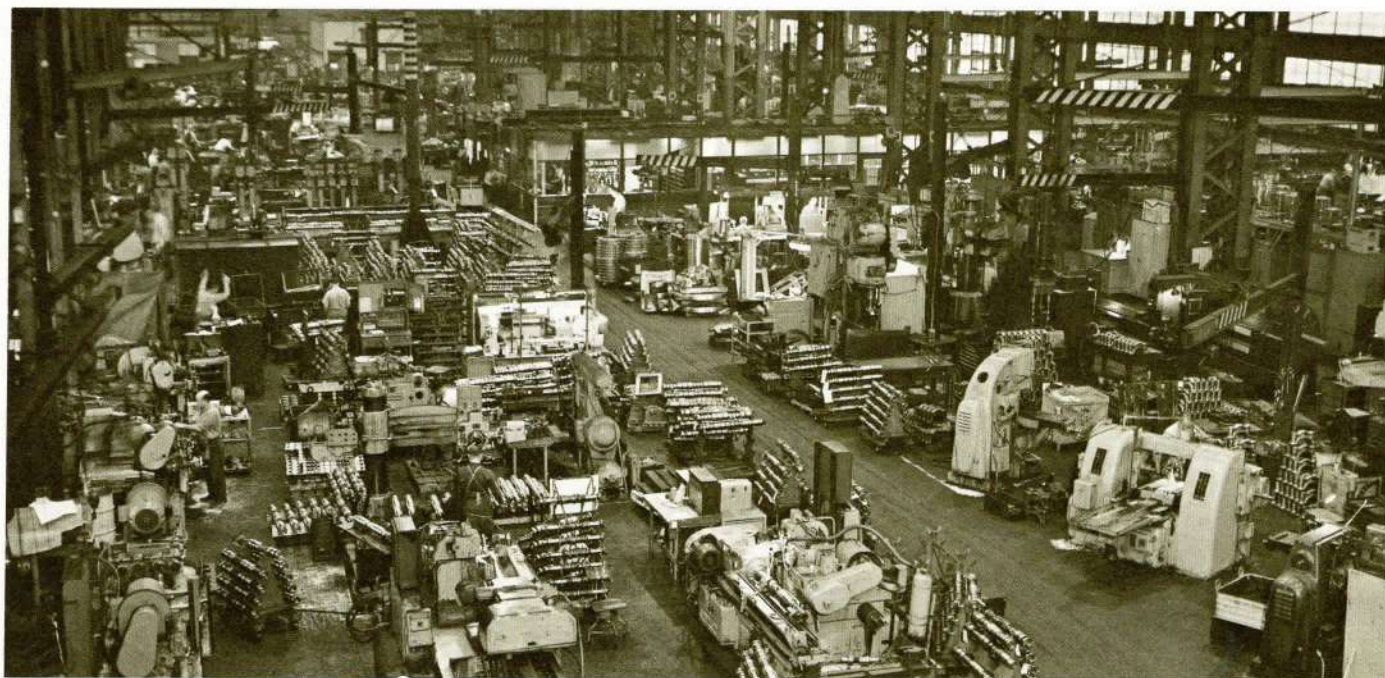
A section of Alco's Auburn, New York plant, where Alco 251 engines for use in locomotives, as well as for diverse stationary, marine and government applications, are assembled.
