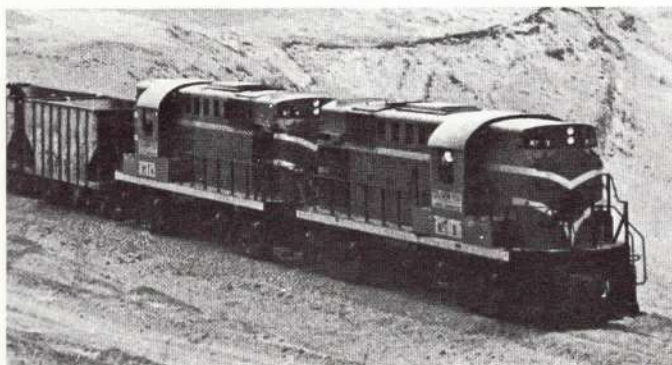
Two ALco DL-701 locomotives haul long copper mineral train on the lines of Southern Peru Copper Corp., at 10,000 ft. altitude.
