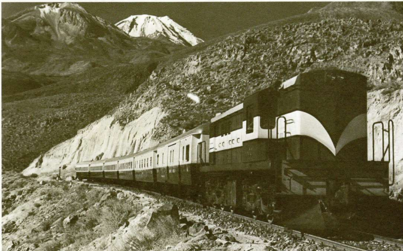
Alco DL-531 unit hauling a passenger express across the Peruvian Andes at 14,688 feet above sea level. Other ALco units operate efficiently in Peru at altitudes in excess of 16,500 feet.
