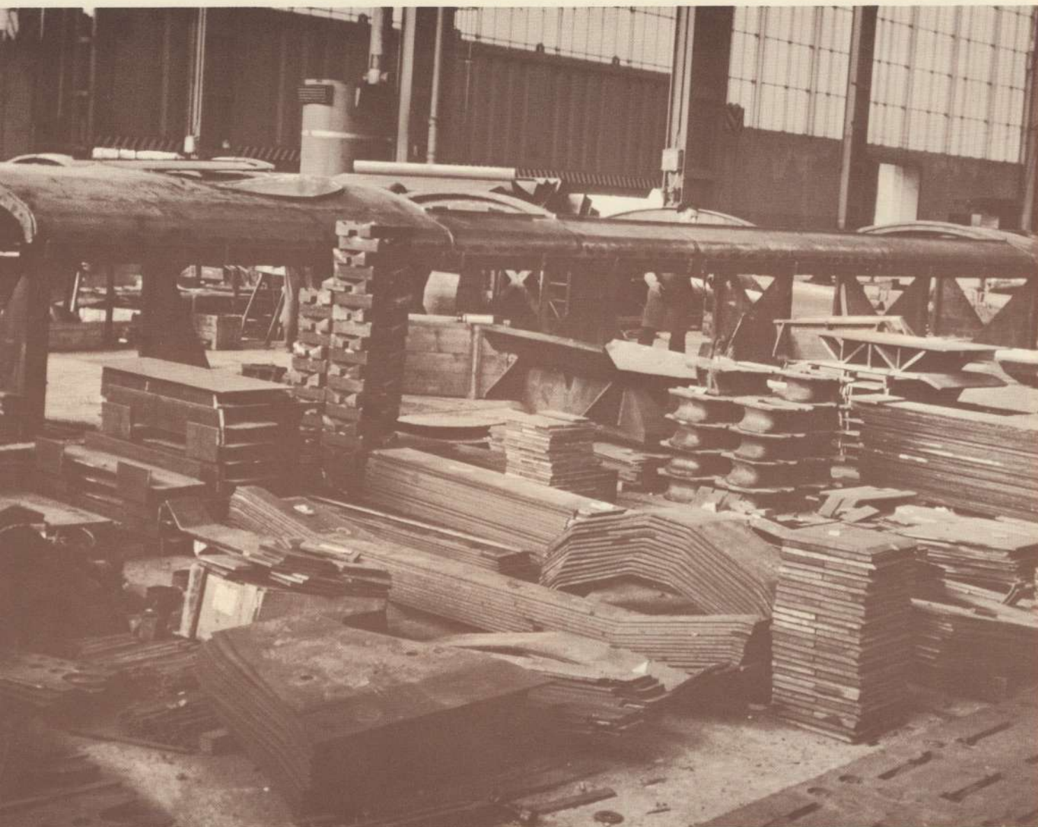
Construction components, pre-fabricated at other locations in the plant, are stored ready for use on the locomotive assembly line at C.A.F.
