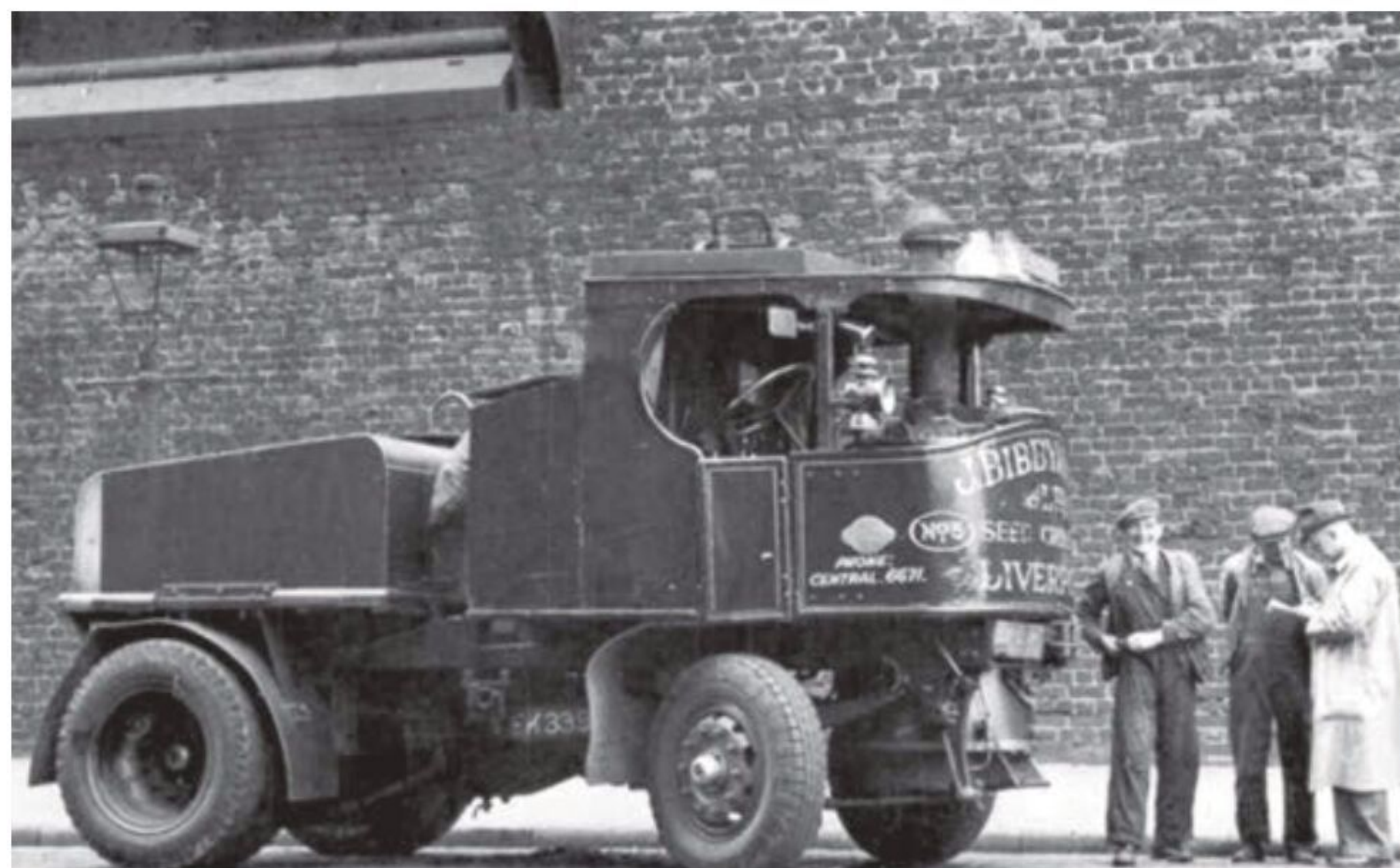
Fig. 10. 4-ton tractor No. 410 converted from a 6-ton wagon. The crew appear to be getting their delivery instructions from the gaffer.
