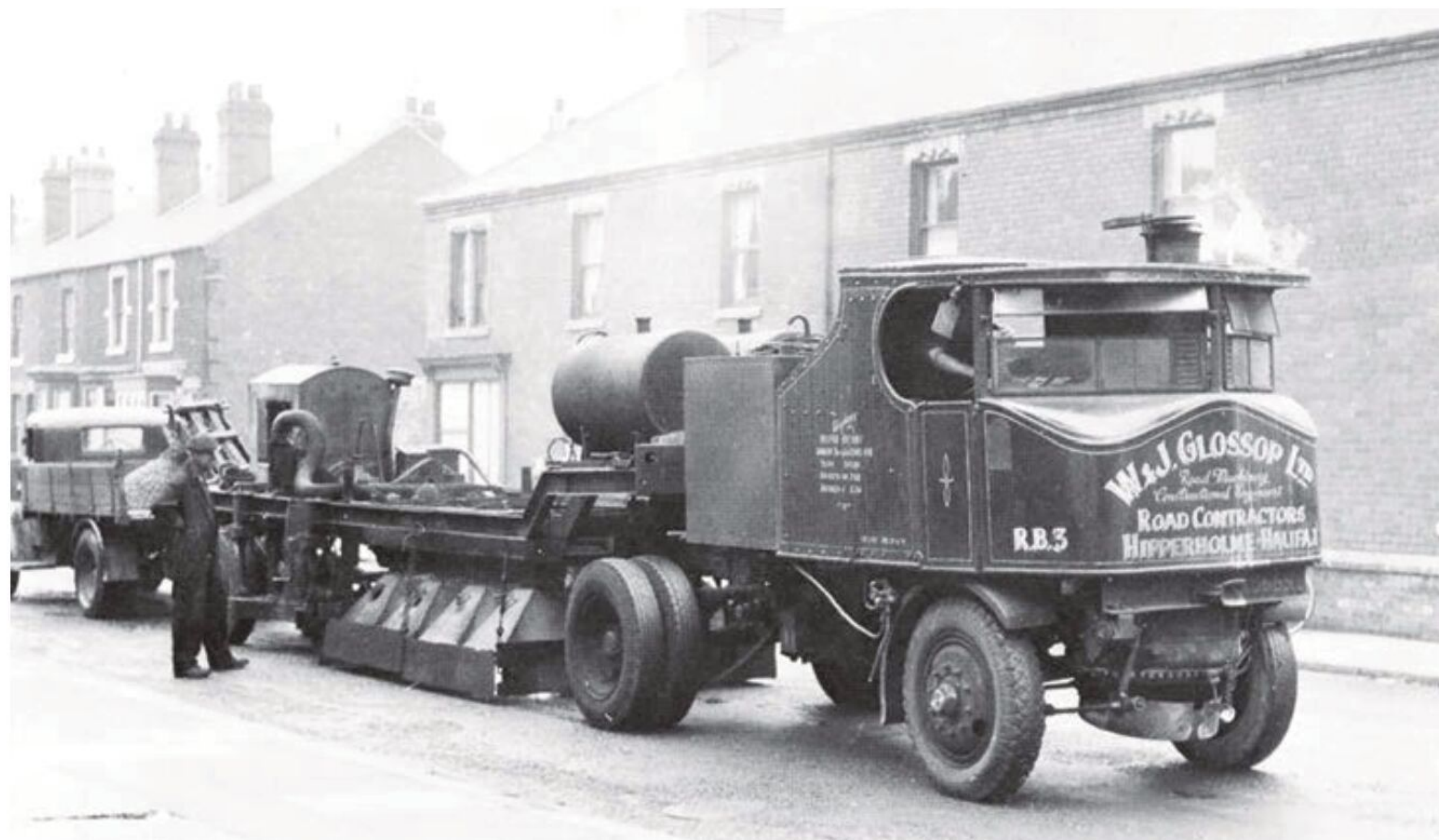
Fig. 3. Super Sentinel No. 6400, when owned by W&J Glossop Ltd, working as an articulated road resurfacing vehicle.
