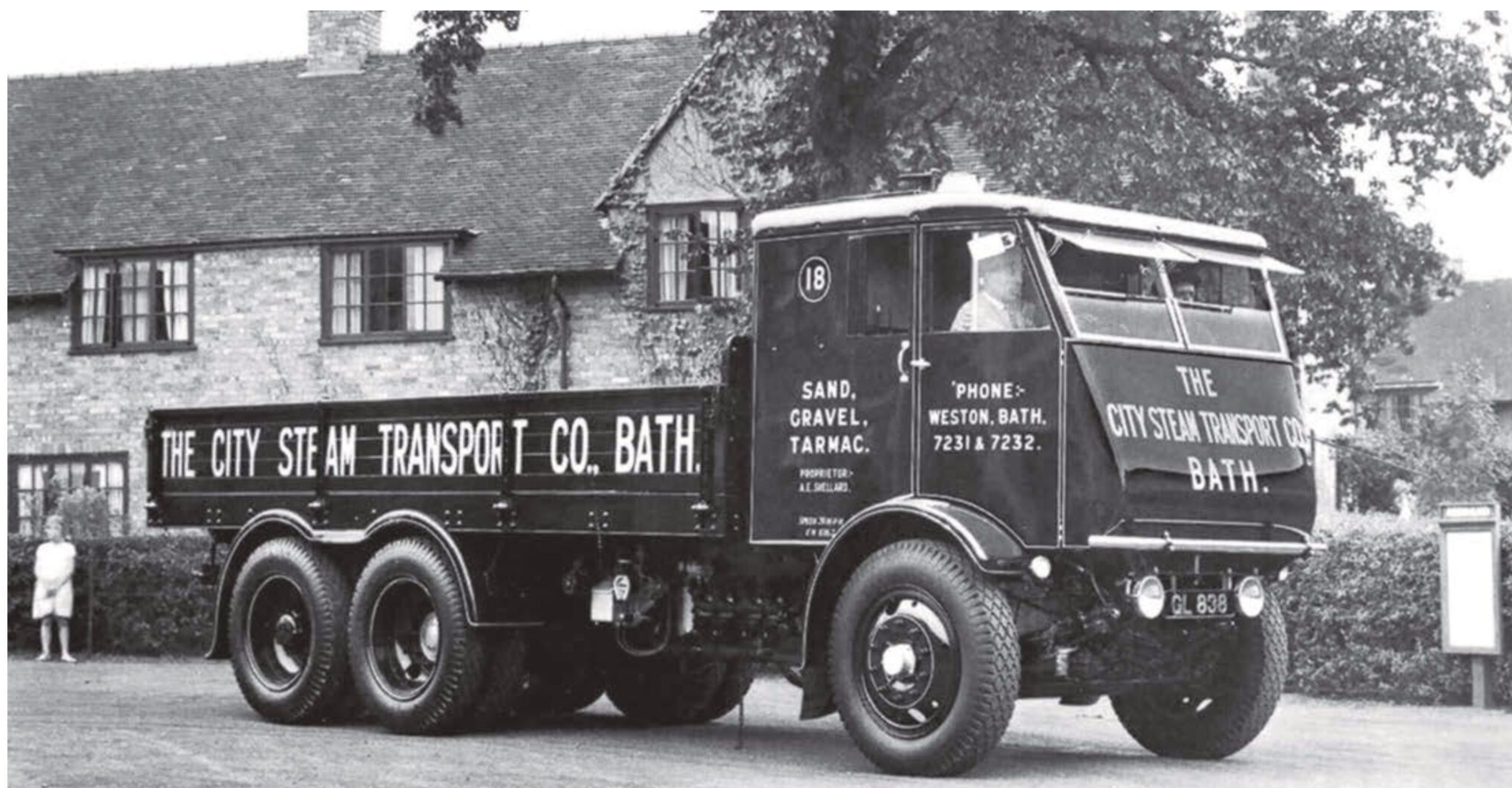
Fig. 7. S6 waggon No. 8849 of 1933 photographed prior to delivery to the customer – not a municipal public transport undertaking as the name suggests, but purveyors of sand, gravel and Tarmac!
