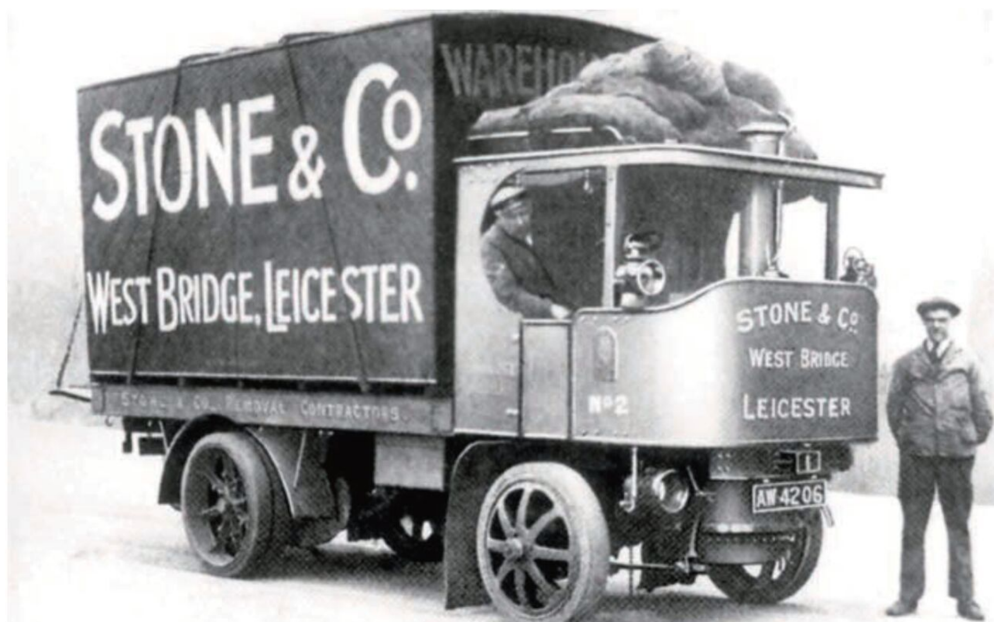
Fig. 5. Sentinel Standard undertype waggon No. 2022 (AW 4206) was built in July 1918 and sold to Stone & Co Ltd of Leicester, where it became No. 2 in their fleet.
