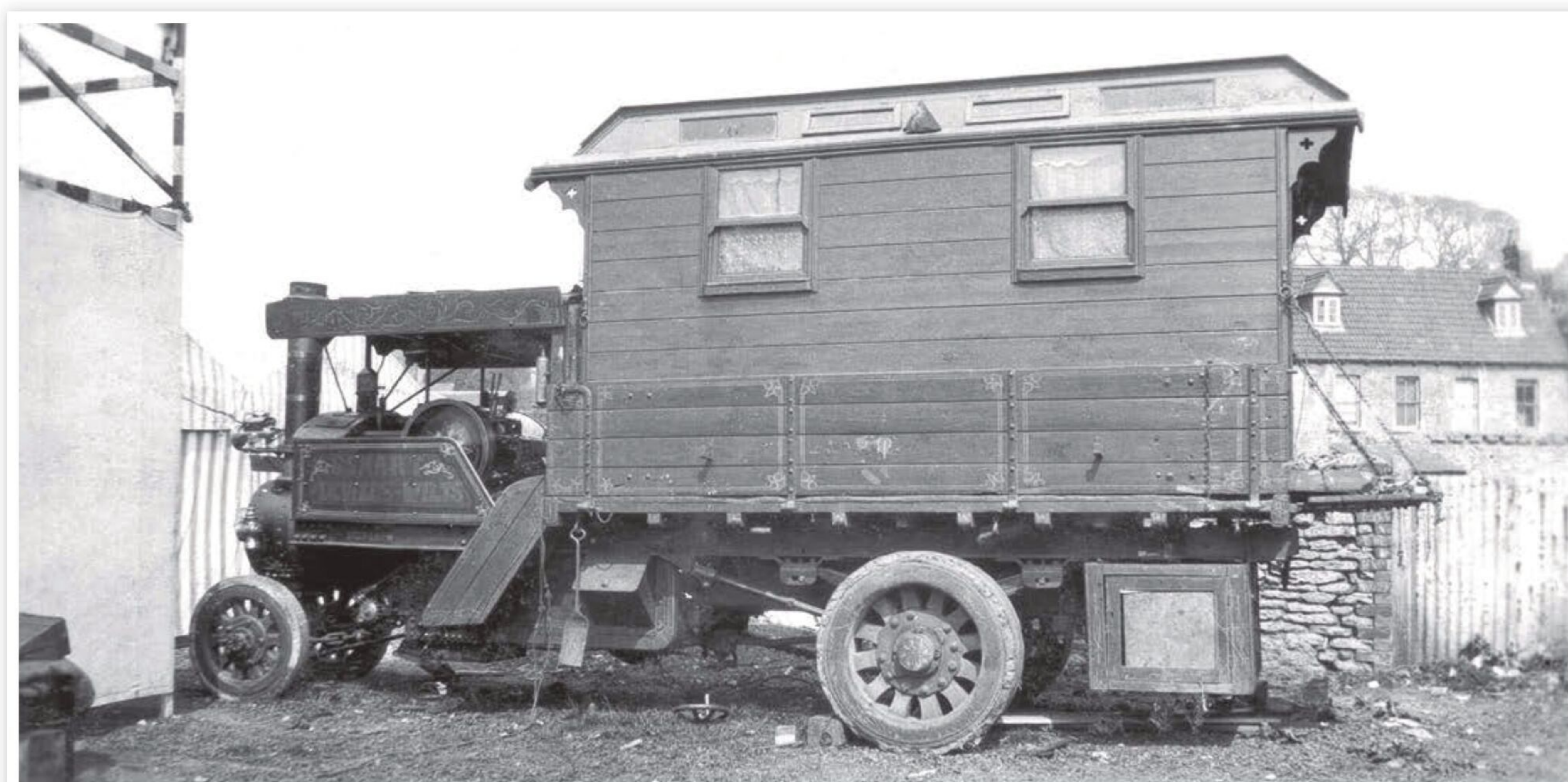
Fig. 8. Wagon No. 47250, carrying a caravan body. This was quite a good idea as it enabled the showman to put the wagon to good use in the winter months, such as delivering coal.
