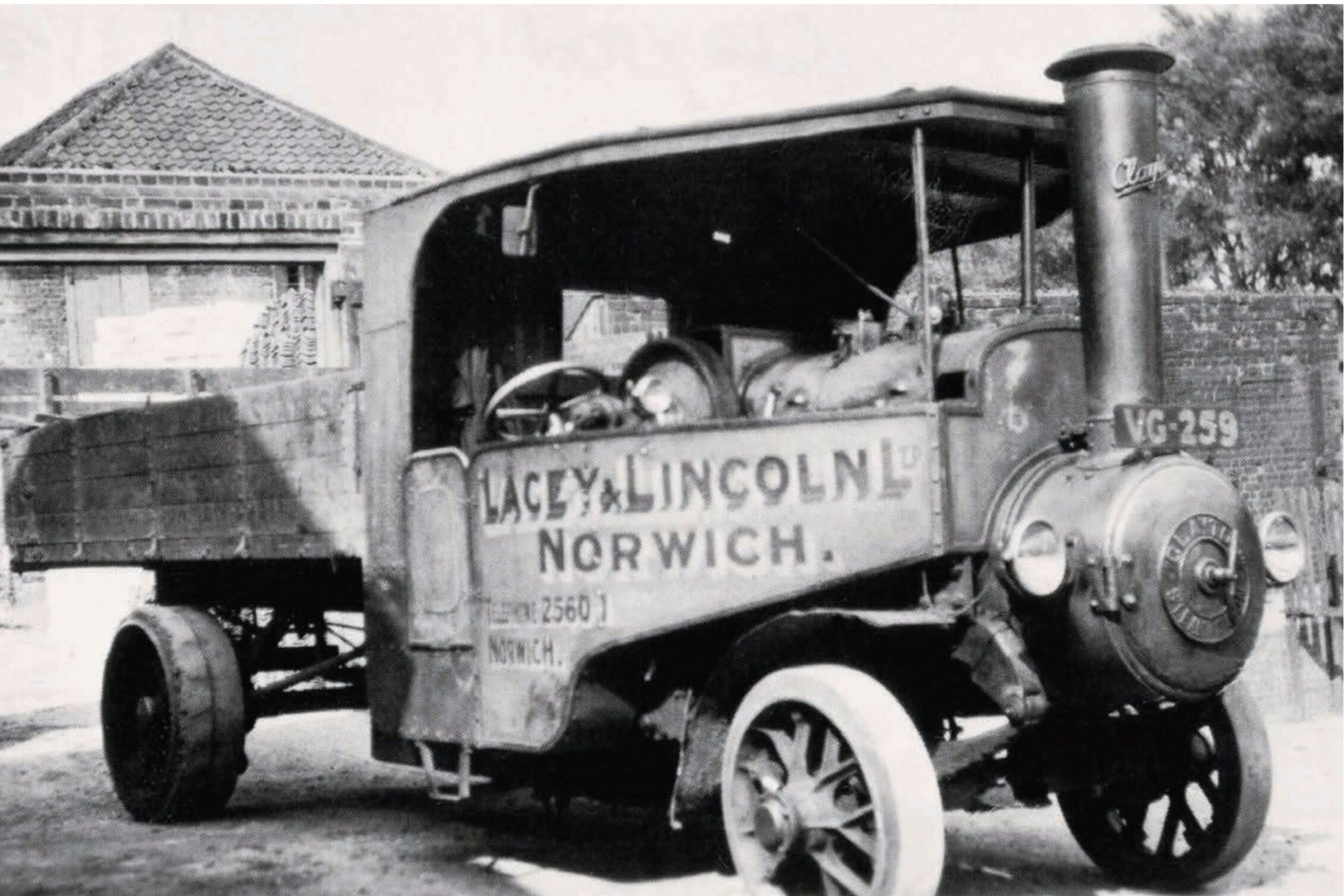
Fig. 7. 6/7-ton 3-way tipping wagon No. T1182 is seen towards the end of its life, photographed in the owner's yard at Norwich on August 28, 1934.
