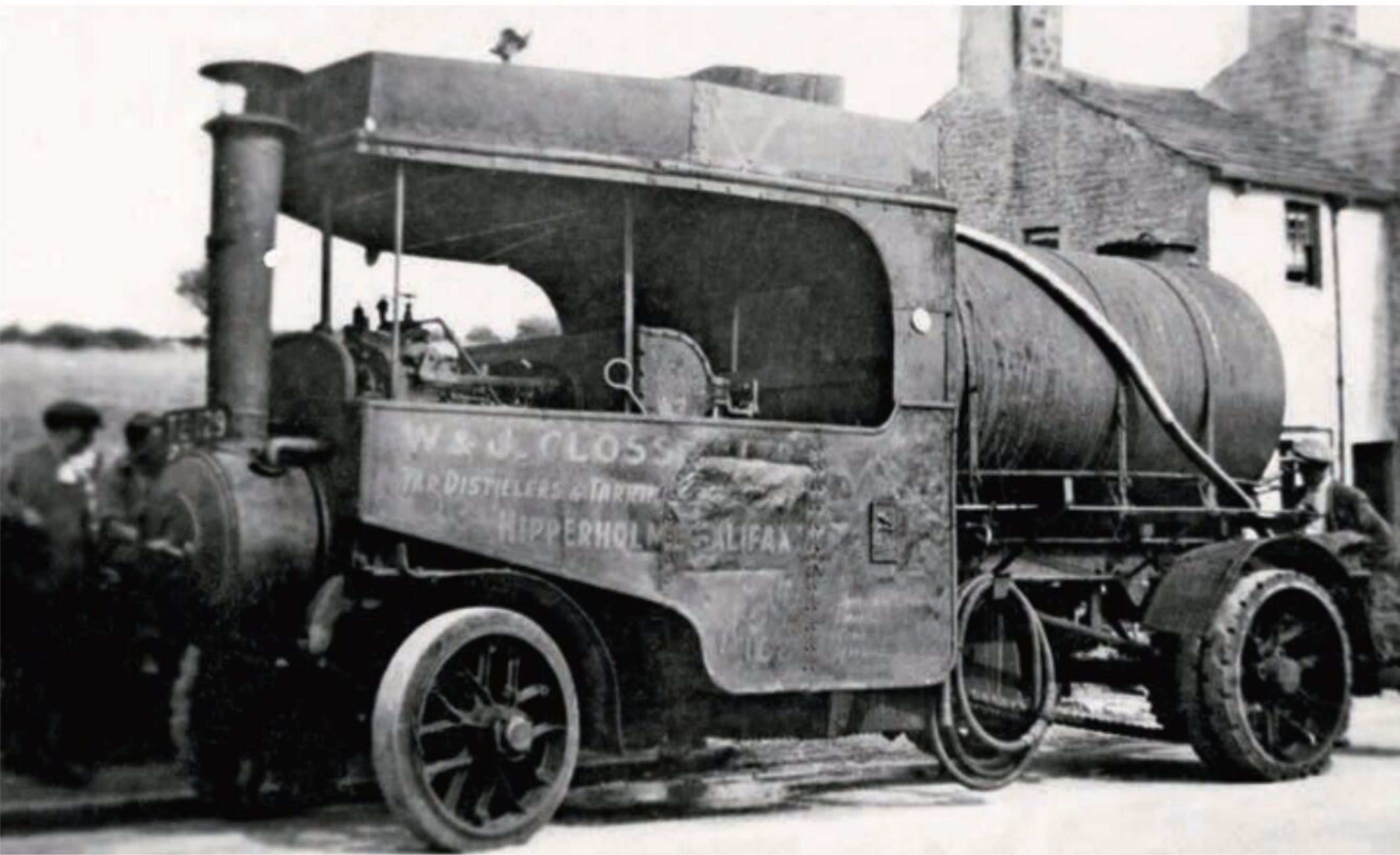
Fig. 6. No. T1148 fitted with tar-spraying equipment on her original short tipper chassis.
