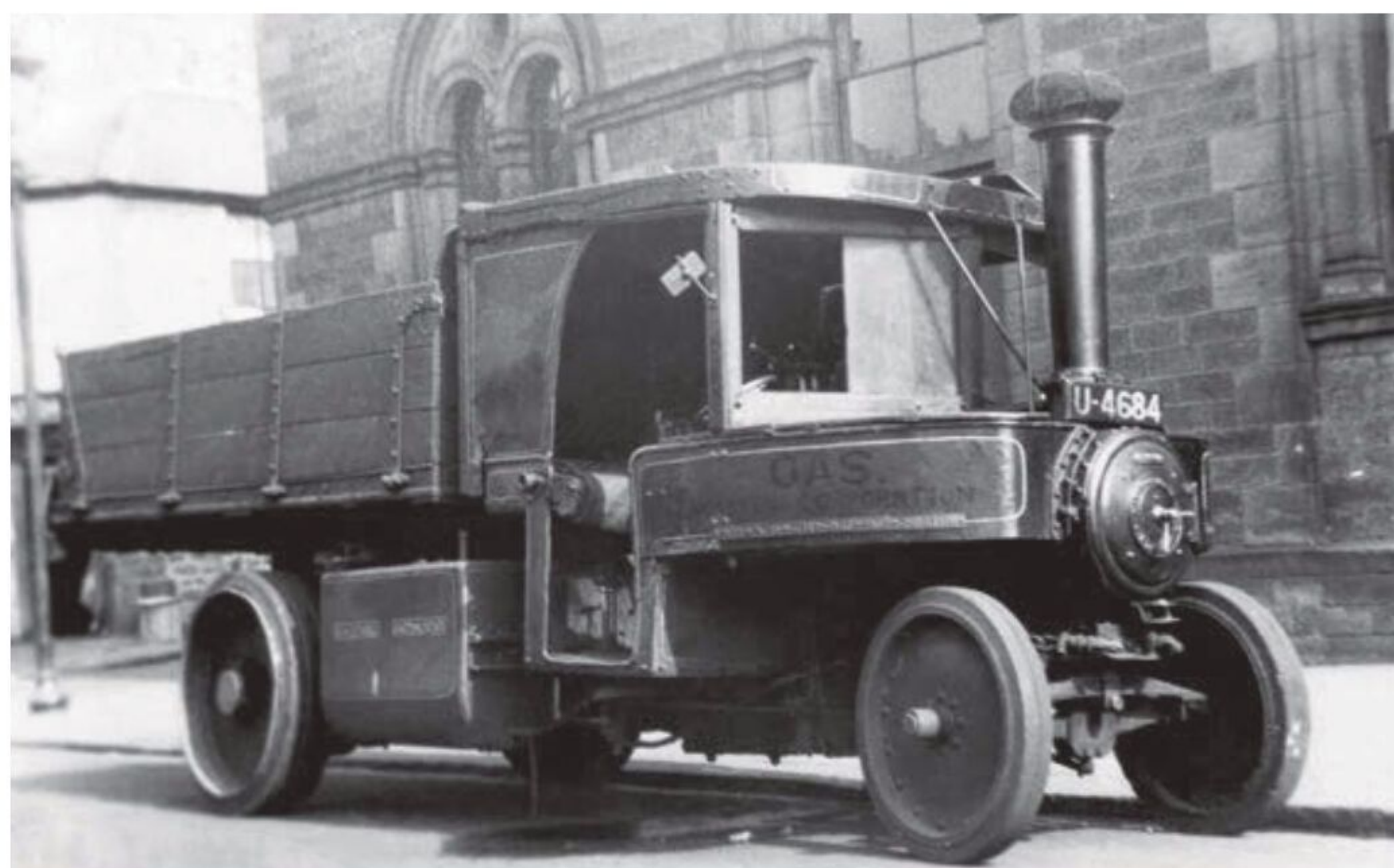
Fig. 6. Four-ton tipping wagon No. 1337 with what appears to be a do-it-yourself windscreen – no glazing but a means of blanking off parts of it when the rain is blowing in.
