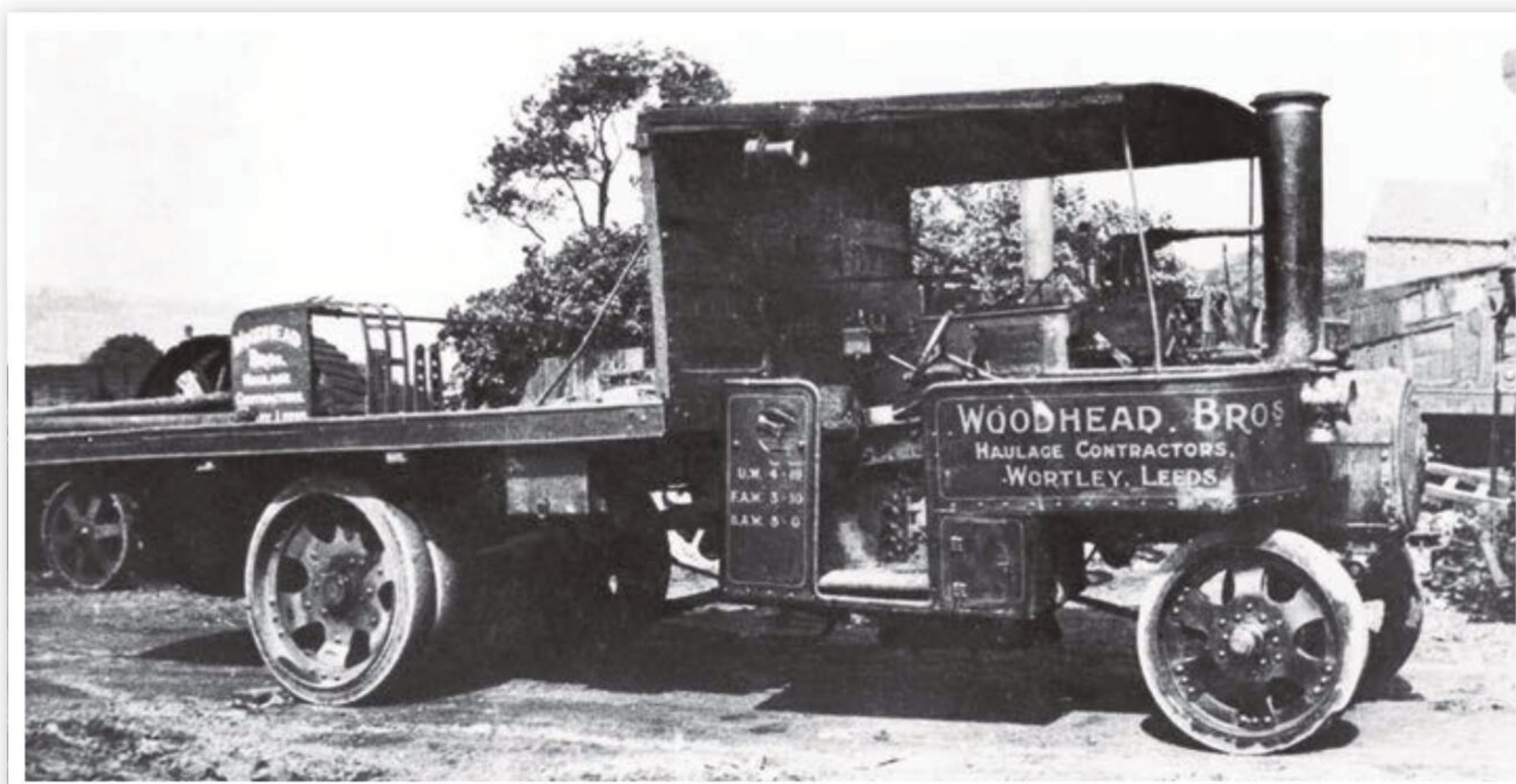
Fig. 3. Mann 4-ton wagon No. 627, a handsome looking vehicle but it appears to have had a working life of only 14 years or so.
