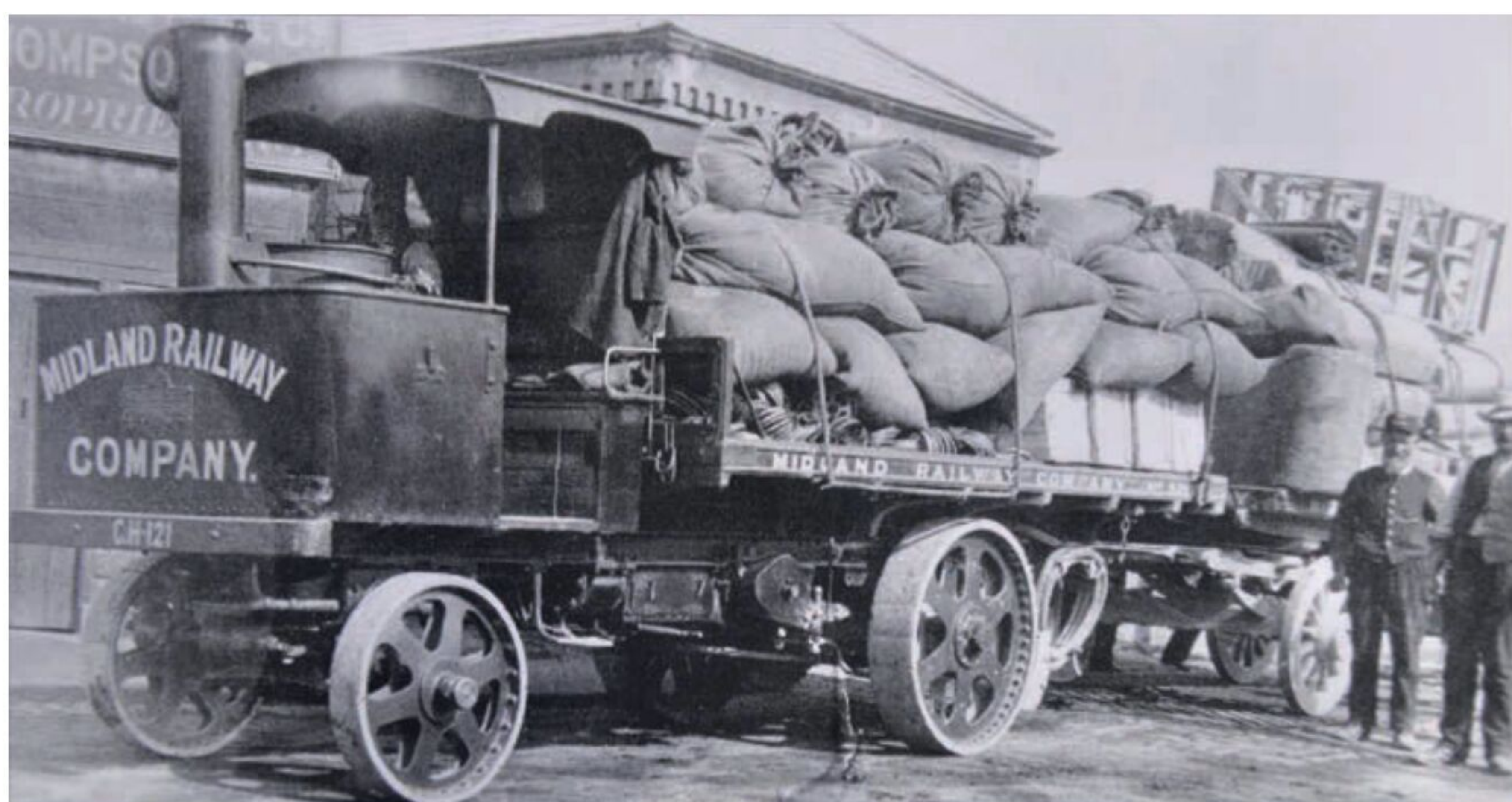
Straker 5-ton wagon No. 120 Reg No. CH 121 built in April 1904 and sold to the Midland Railway Co for use at their Bath Goods Depot, receiving their fleet No. 5263. These wagons had the power to pull a trailer carrying a load of 2 tons, giving a respectable payload of 7 tons, which was very good bearing in mind the unmade roads of the day.
