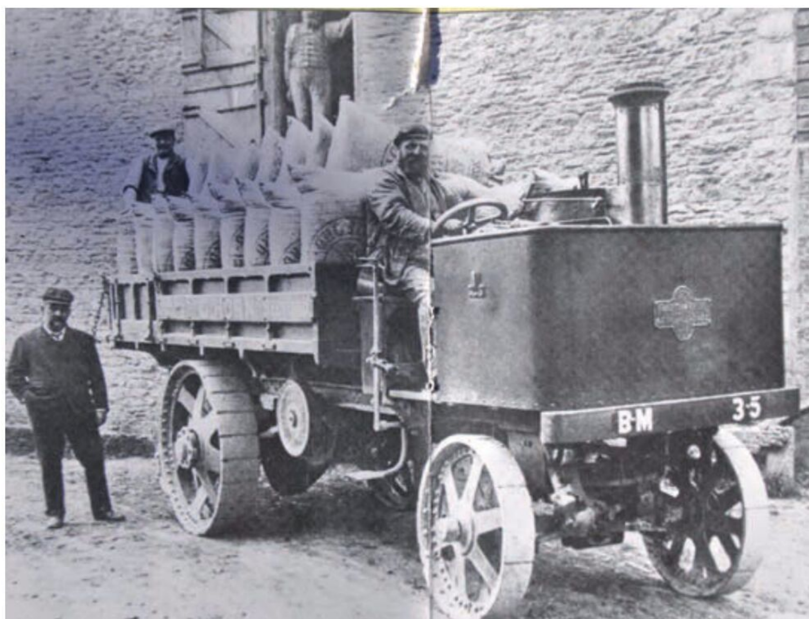
Straker 5-ton wagon No. 120 Reg No. CH 121 built in April 1904 and sold to the Midland Railway Co for use at their Bath Goods Depot, receiving their fleet No. 5263. These wagons had the power to pull a trailer carrying a load of 2 tons, giving a respectable payload of 7 tons, which was very good bearing in mind the unmade roads of the day.
