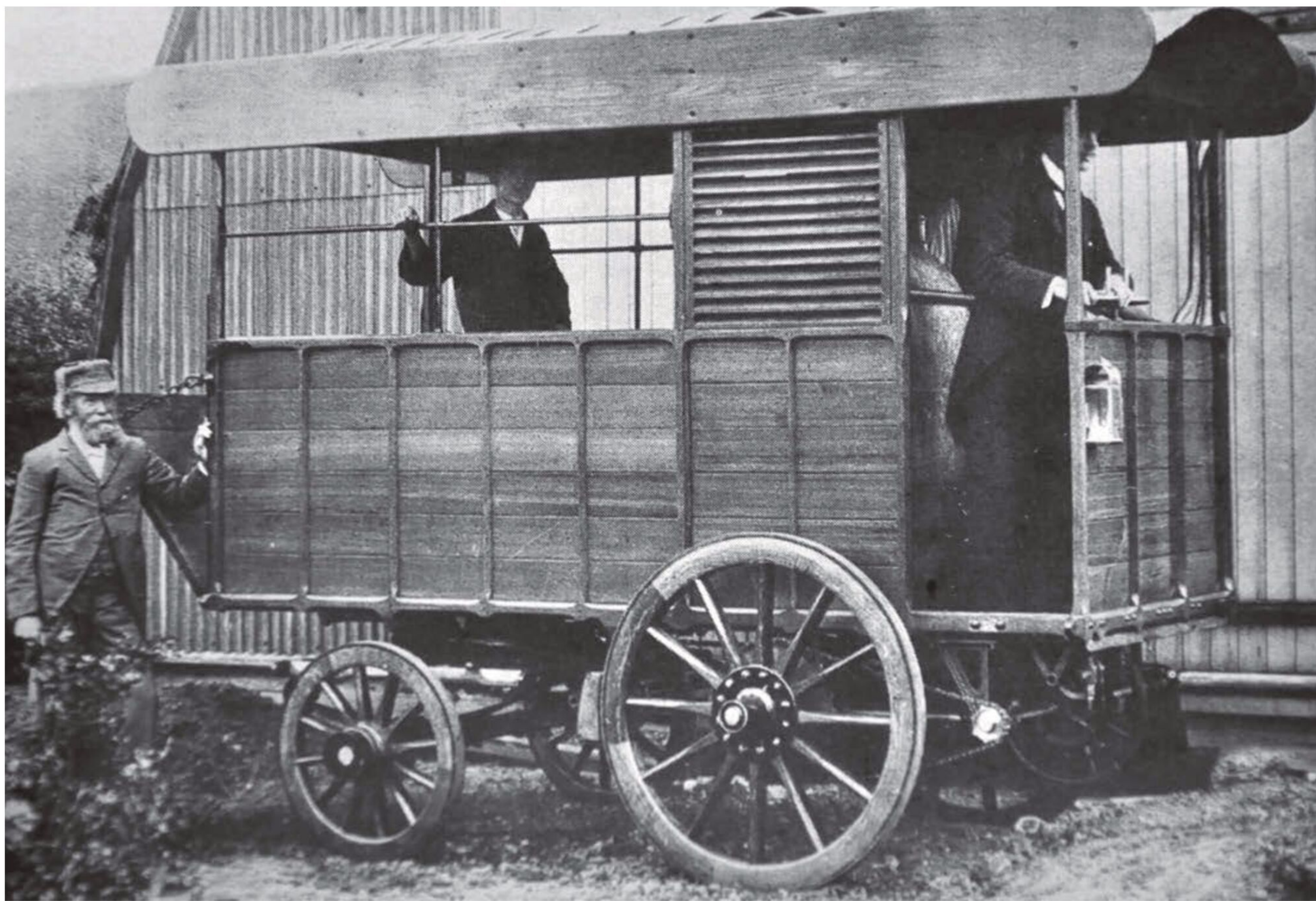
Thornycroft No. 1. This 1-ton van, built in 1896, was the company's first venture into the newly-emerging commercial vehicle business. Heavy gears and chains were just not available, hence the very frail-looking chain drive to each front wheel. The steering operated on the rear wheels. John Thornycroft stands to the left of the photo, little realising where his experimental wagon would lead his company.
