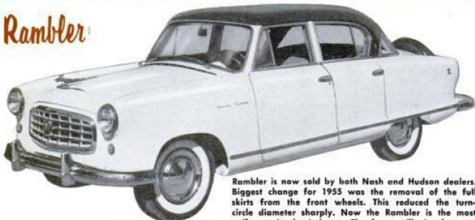
Rambler is now sold by both Nash and Hudson dealers. Biggest change for 1955 was the removal of the full skirts from the front wheels. This reduced the turn-circle diameter sharply. Now the Rambler is the most agile car in the industry. The front grille is also new
