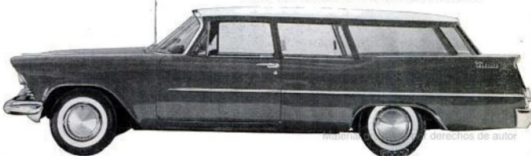
Plymouth wagons have a locked compartment in rear for valuables. Spare tire and gas tank are mounted within rear fenders. The third seat faces rearward
