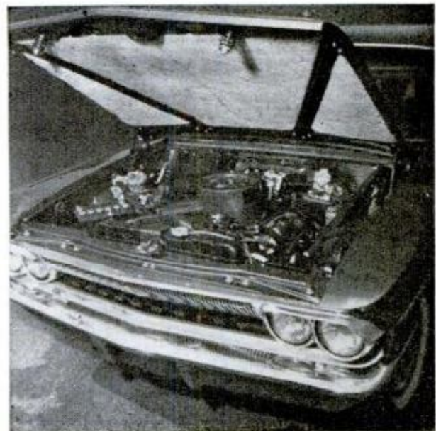
Broad hood swings up to reveal F-85's engine which has "most serviced" items easy to reach
