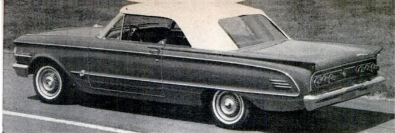
COMET , like its companion compact Falcon, gets a convertible for '63. On 114-inch wheelbase, it will have power operated top, bucket-type front seats and a choice of the 85 or 101-horsepower six-cylinder engines
