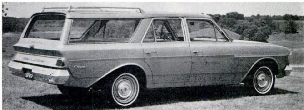
STATION WAGONS have all-new bodies too, but there's still a trace of the dipped roofline that's been a Rambler wagon trademark since 1955. The three-seat model, above, continues to use a swing-out rear door
