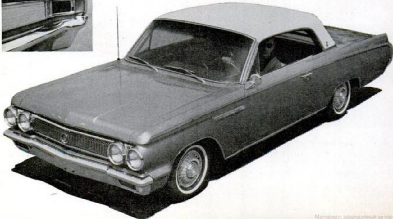
BUICK SPECIAL has rear quarter panels (left) that extend four inches beyond actual end of car to add unusable length. Skylark sport coupe is shown below
