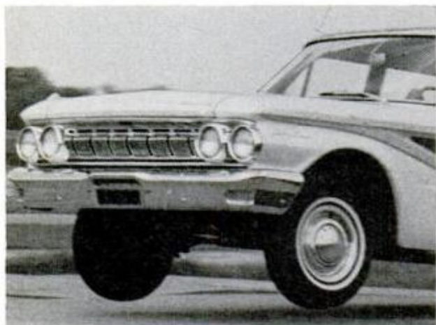
METEOR takes to the air, but two-way stretch of its "compliance" front suspension helps soak up shock
