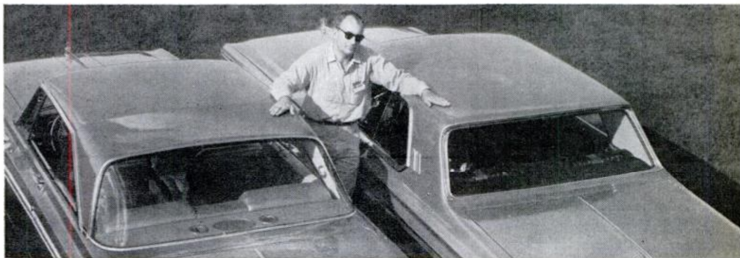
PROGRESS IS SOMETIMES MADE by going backwards, and the '64 Plymouth two-door hardtop, left, with its curved backlite much like 1960-61 Plymouth's, is a perfect example. The 1962-63 window, right, restricts rear vision at corners
