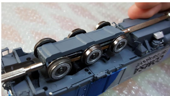
5. Use a second screw driver to avoid the closing on the other side. Now lose the other remaining 3 snap-fits and the cover should com of easily
