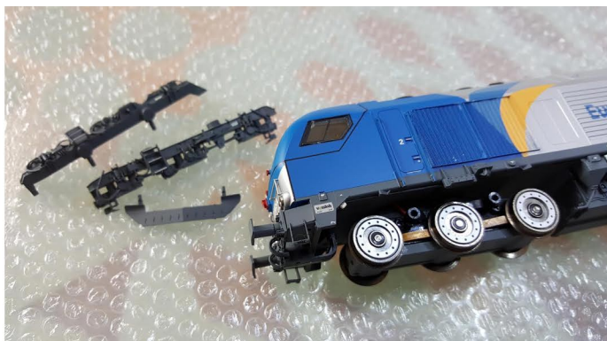
1. Remove front skirt and bogie/truck sides (just pul them out, there are not glued)
